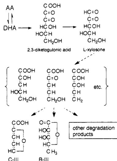
**Figure 5.** Tentative scheme for the degradation of DHA.
