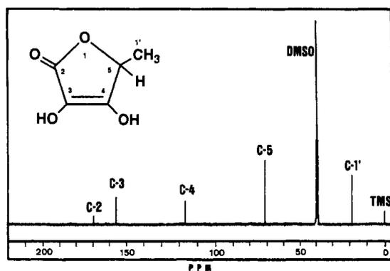
**Figure 3.** Proton-decoupled  $^{13}C$  NMR spectrum of brown pigment B-III and its chemical structure: 3,4-dihydroxy-5-methyl-2(5H)-furanone.
